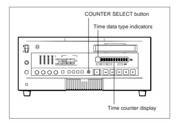
Press the COUNTER SELECT button on the front panel of the unit.
